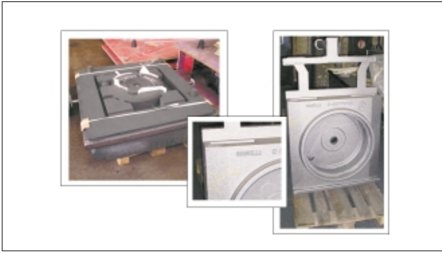
Figure 10. Milled sand mould (left) for cast prototypes (right)
